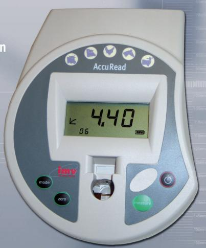
Small and portable sperm cell density meter, Accuread operates on AC and battery. Direct reading of concentration through long life LED source combined with fibre optic (no filter). Also displays results in direct concentration or absorbance. RS 232 plug enables printing.
